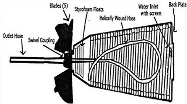
Fig. 1 Inner workings of the Rife River Pump.
